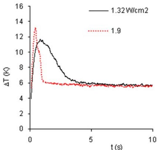
**Fig. 6** Evolution of overheating in the small zone of nucleated boiling.
