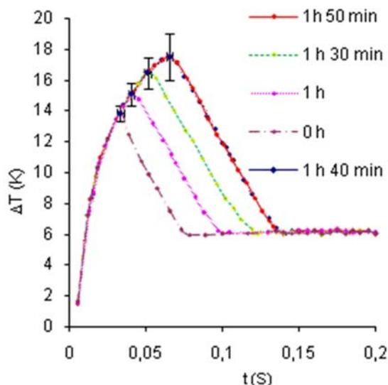
**Fig. 10** Temporal evolution of overheating for different time-delays for a horizontally fixed ribbon.
