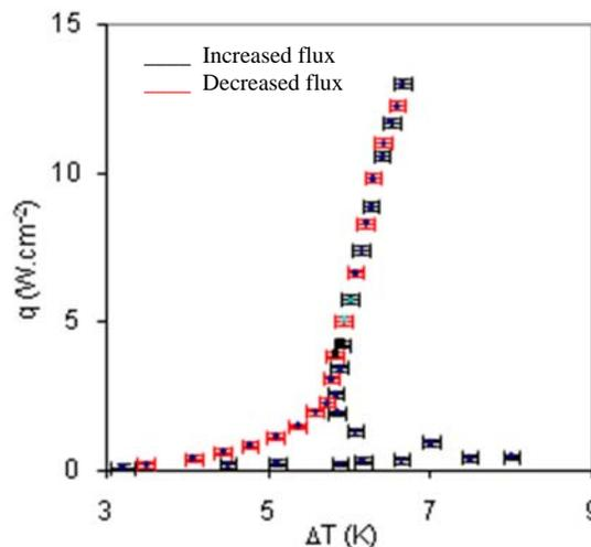
**Fig. 4** Comparison of experimental boiling curves of liquid Nitrogen during steady regime for an increased and a decreased flux in contact with a horizontally fixed ribbon at saturation under a pressure of 1 atm.
