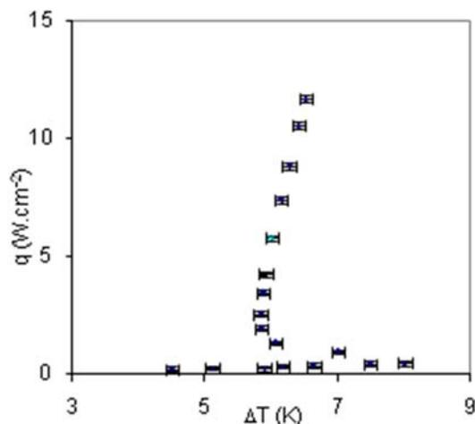
**Fig. 3** Boiling curve of liquid Nitrogen in steady regime with an increased flux in contact with a ribbon mounted in horizontal position at saturation under a pressure of 1 atm.
