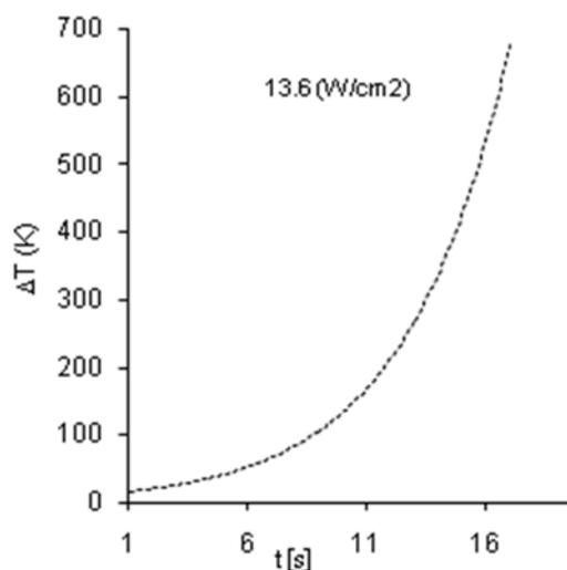
**Fig. 9** Temporal Evolution of overheating. The flow pulse begins at  $t = 1$ sec and lasts at 20 sec.
