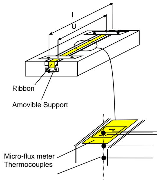
Fig. 2 Experimental Set-up for a ribbon horizontally positioned.
