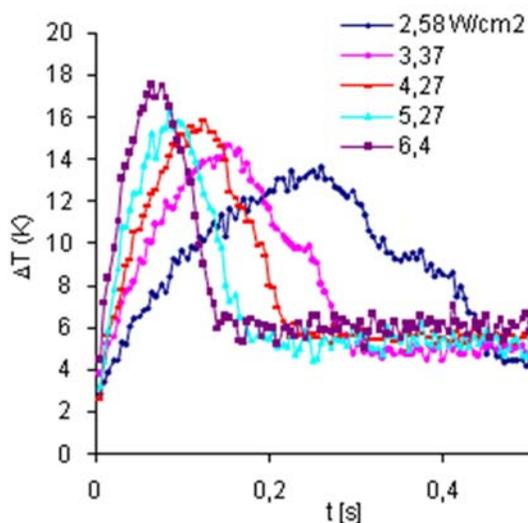
**Fig. 7** Overheating in the nucleated boiling zone fully developed.
