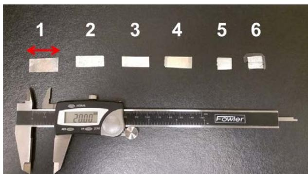
**Fig. 10** TIM samples. The red arrow represents the CTE measuring direction.
