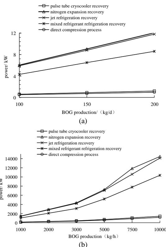
Fig. 1 Power Consumption Comparison of BOG Processing Technology in LNG Station
